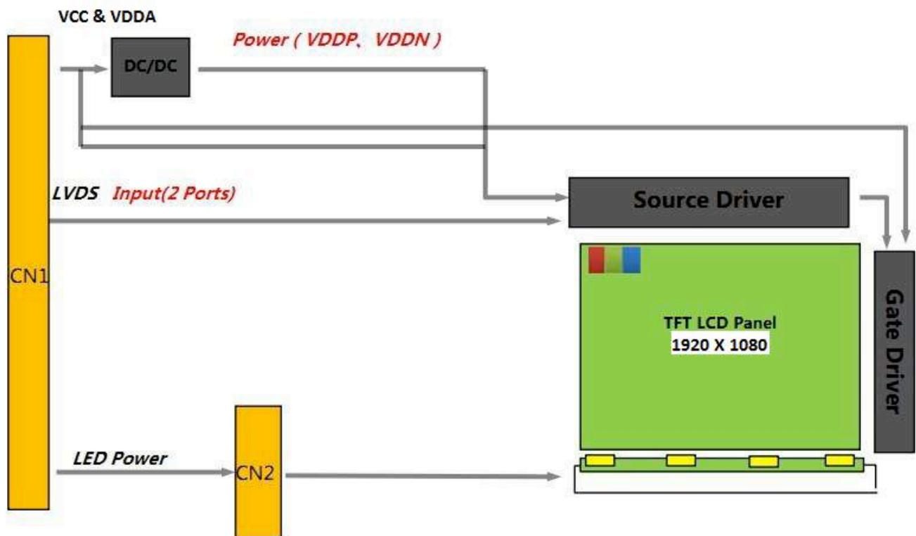
Figure 1: Function Diagram
