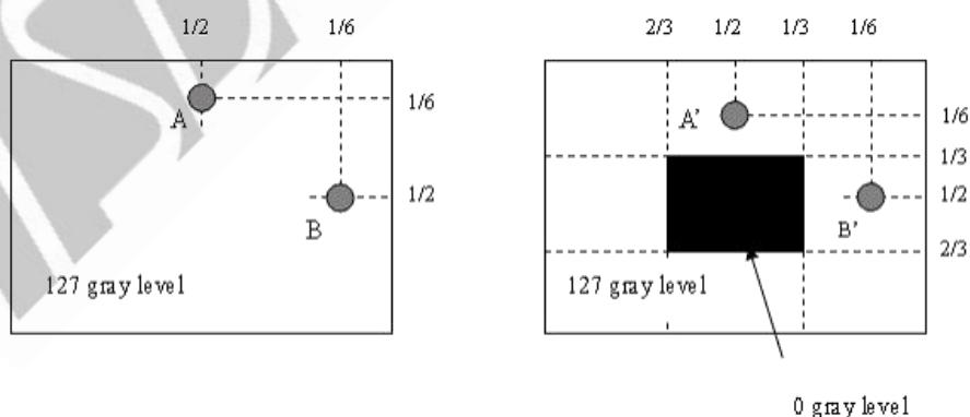
$1 \text{ LA-LA}' / \text{LA} \times 100\% = 2\% \text{ max.}$ , LA and LA' are brightness at location A and A'.
